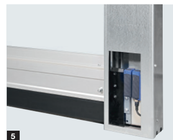
SC 1500 SEL 2.0 MP MACHINE PROTECTION Thanks to the safety sensors the door can open only when the machine is idle and the machine can be operated only when the door is closed.
